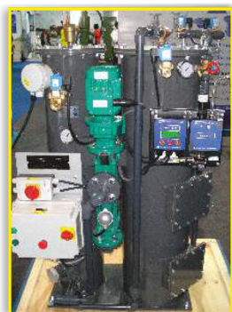
Roto Pump feeding oily water on OWS
